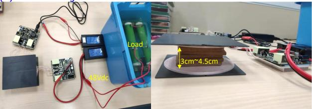
(2) As a battery charger: Directly charge a 48V battery
